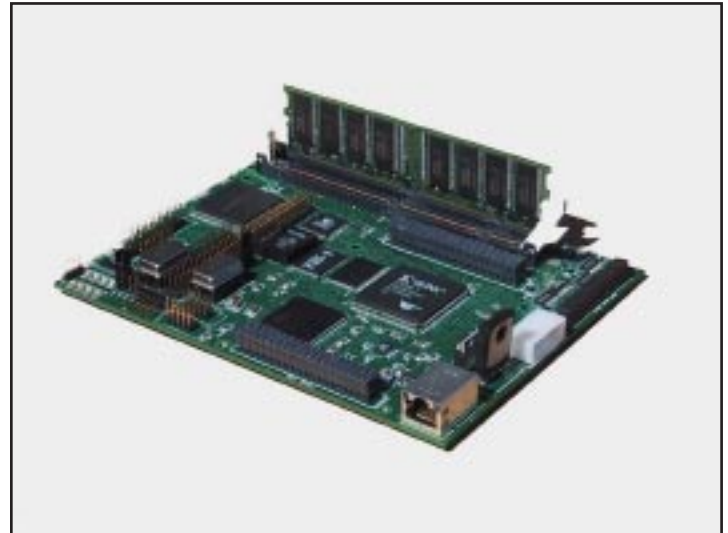
The ESP-1 Embedded System Platform is shown with one SDRAM DIMM installed.
