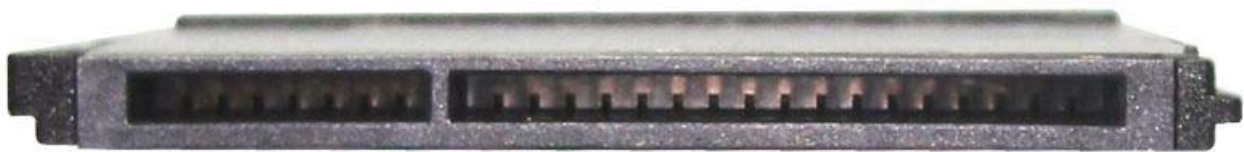
Figure 4: SATA 7-pin (data) + 17-pin (power)
